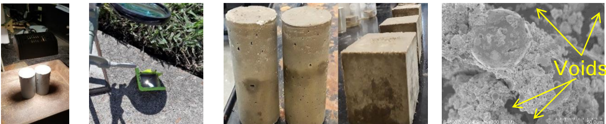
Figure 1: Curing FPGPC Samples, Cured Cylinder and Cubes and SEM Image Showing Unreacted Components
