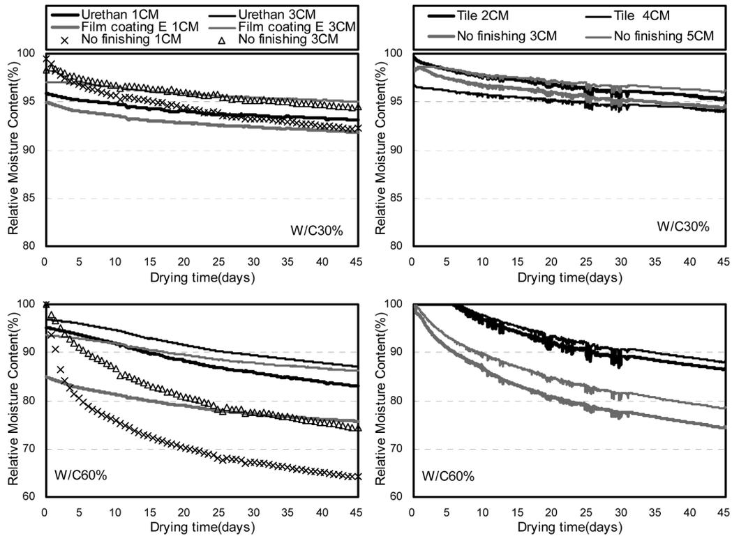
Fig. 5 Time-related changes in the RM distribution in coated/tiled concretes under drying.
