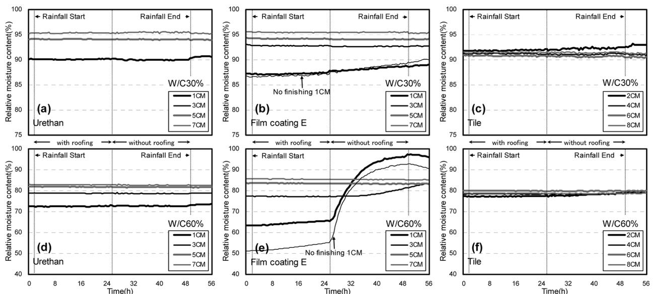
Fig. 10 Time-related changes in the RM distribution in coated/tiled concretes with and without roofing.
