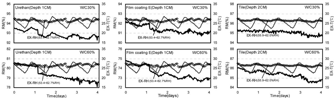
Fig. 7 Time-related changes in the RM distribution in coated/tiled concretes under cyclic temperature changes.
