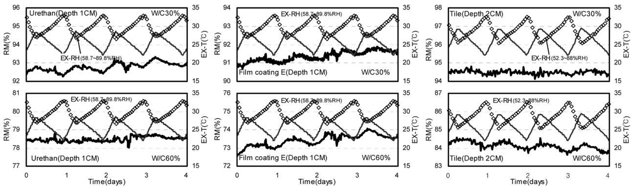
Fig. 8 Time-related changes in the RM distribution in coated/tiled concretes under cyclic temperature-humidity changes.
