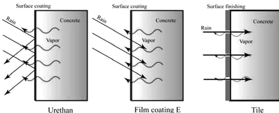
Fig. 12 Schematic expression of the water permeability of finishing materials.
