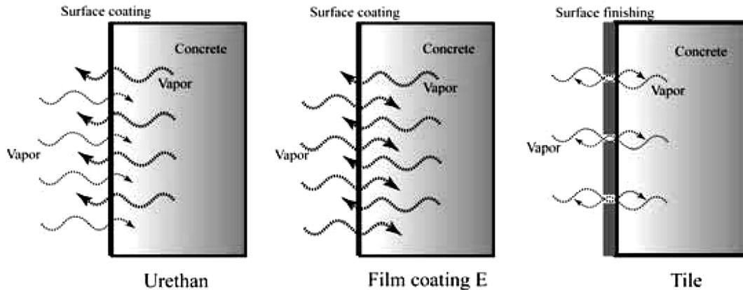
Fig. 9 Schematic expression of the vapor permeability of finishing materials.
