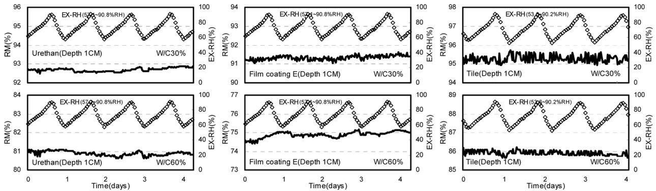
Fig. 6 Time-related changes in the RM distribution in coated/tiled concretes under cyclic humidity changes.
