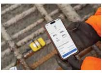
cracking. It is fully wireless, with an embedded sensor that measures the internal temperature and determines strength of a concrete placement. The Signal Sensor, easy to install and instantly connected to a ConcreteDNA dashboard, equips field teams with real-time data anywhere. The DEWALT Signal Sensor is available at White Cap.
