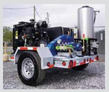
can also be used as a standard waterblasting unit by bypassing the heater. The 2000 Series Hot Water Unit features a purpose-built control panel and pressure control devices, as well as an onboard 90 gal. (341 L) water tank and charge pump that ensures a consistent water supply. The hot water system is mounted on a low-profile 5000 lb (2268 kg) trailer, with a galvanized steel frame to prevent corrosion and a properly rated torsion axle to minimize suspension wear.
