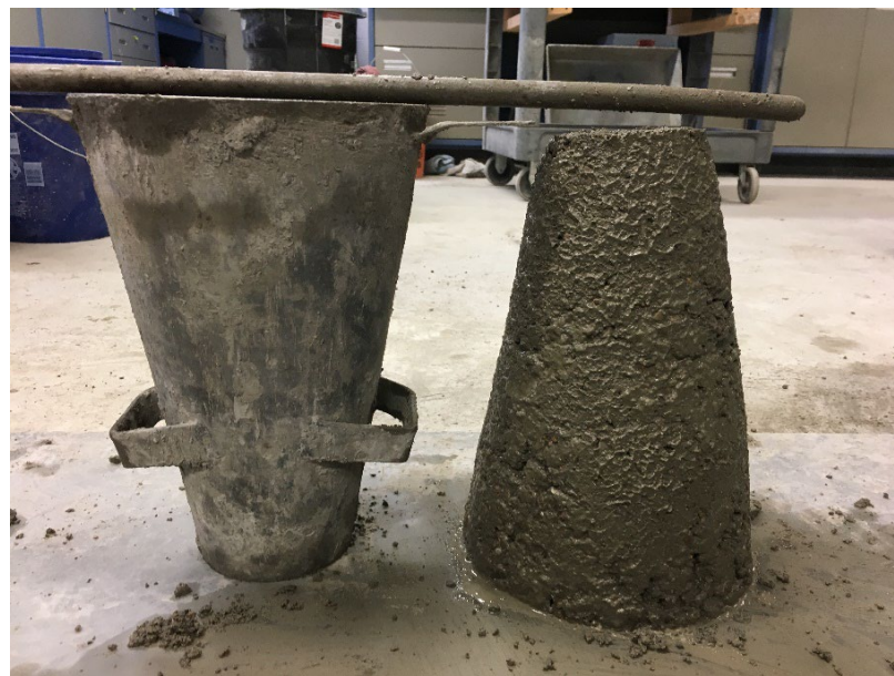
Figure 29 Slump test setup
