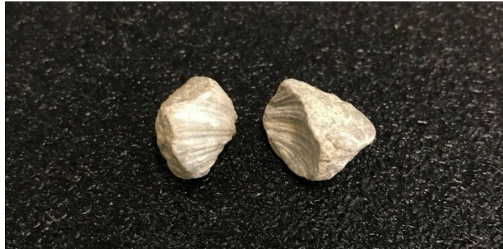
Figure 20 Example of natural aggregate becoming too brittle
