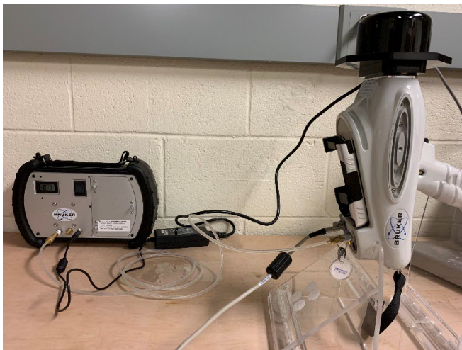
Figure 27 PHXRF connected to a vacuum pump
