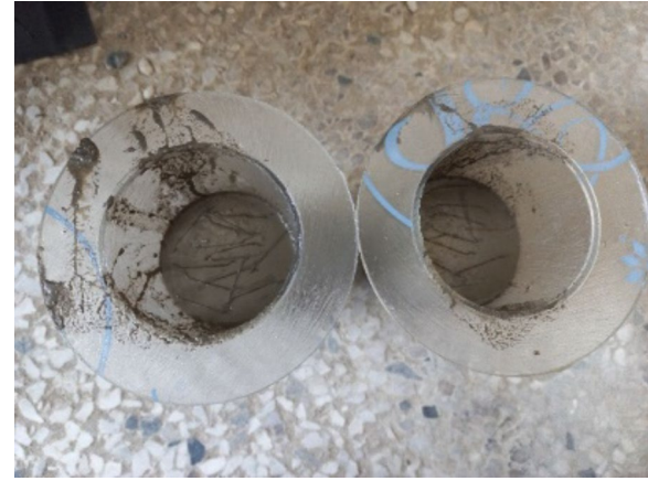
Fig. 5 Steel fiber placement
