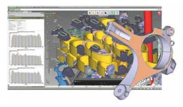
graphic files to represent the geometry in detail regardless of the size of the part. The 4D\_Additive build processor can generate exact slicing curves for printing processes such as selective laser sintering (SLS) and selective laser melting (SLM). By using exact CAD models for slicing and SVG files with exact image resolution, the information on the individual material layers is sent to the printer with very high precision and without loss of quality.
