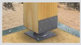
The load-rated ECB can be easily attached to wood framing foundations using Simpson Strong-Tie Strong-Drive® SDS Heavy-Duty Connector screws or anchored into concrete foundations with adhesive or mechanical anchors. The versatile ECB design allows for four-corner-hole installation in wood or single-center-hole installation in concrete.
