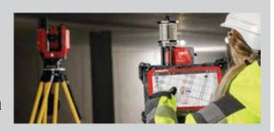
The PLT 400 can be used to lay out projects directly from building information modeling (BIM) data, without the time-consuming need to create points on the plans first. It can also be used during the building process to help keep BIM models up to date, contributing to a highly efficient end-to-end workflow. Hilti's digital construction software is compatible with Revit, AutoCAD, and other professional layout platforms.
