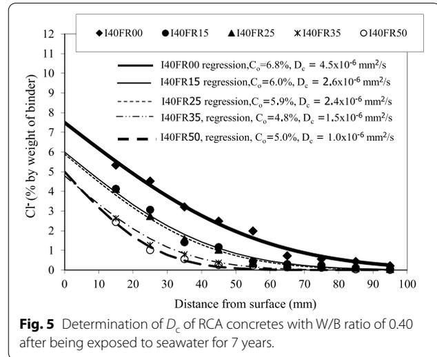
**Fig. 5** Determination of  $D_c$  of RCA concretes with W/B ratio of 0.40 after being exposed to seawater for 7 years.
