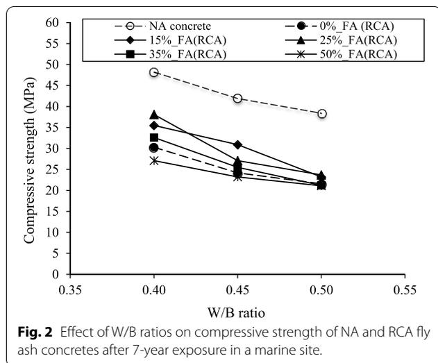
W/B ratio up to 0.50, the compressive strength of the concrete only varies from 21.2 to 23.7 MPa.
