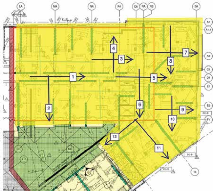
Fig. 1: The yellow shaded area indicates the portion of the podium level slab where 12 sample measurements lines were marked for use in F-number analysis. The lines varied in length from 20 to 35 ft (6 to 11 m). Point coordinates of the start and end of each line were measured using a total station, and these coordinates were provided to each participant. Eight participants performed a laser scan on the lines on two separate days and provided composite F-numbers determined per ASTM E1155 in addition to information on each sample measurement line. For comparison, a Type II device (Dipstick®) was used to collect data twice on the same sample measurement lines
