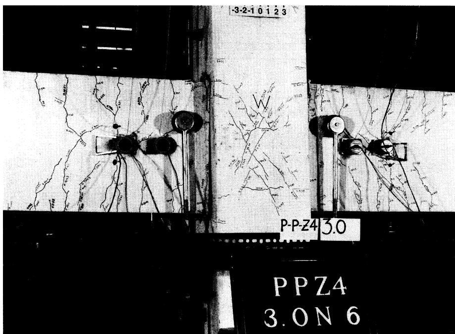
Fig. 24—P-P-Z4 at failure (2.9 percent story drift in aftershock)
