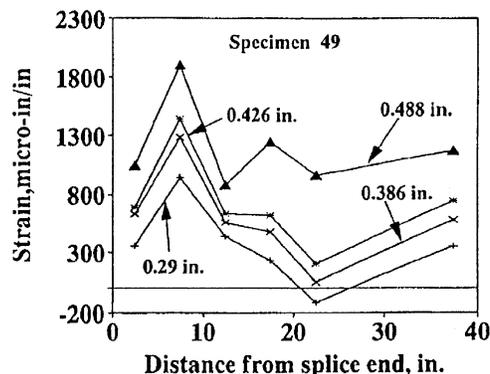
Fig. 11—Strain in stirrups placed over splice region: Specimen 49.
