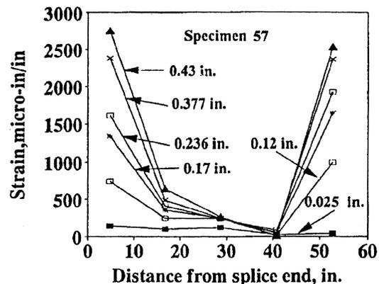
Fig. 9—Strain in stirrups placed over splice region: Specimen 57.
