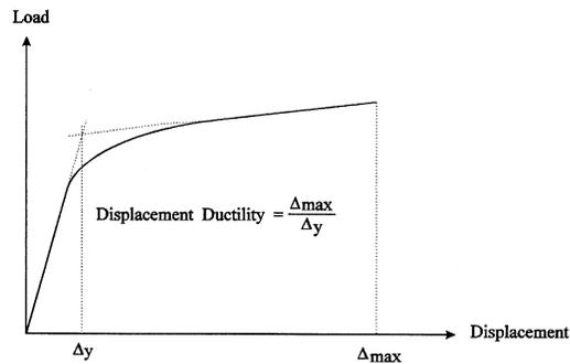
Fig. 6—Definition of displacement-ductility ratio.
