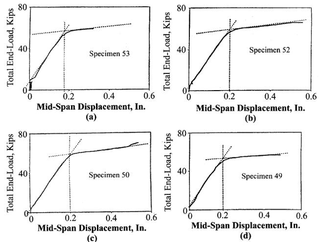
Fig. 8—Load-displacement response of specimens with stirrups: (a) Specimen 53; (b) Specimen 52; (c) Specimen 50; and (d) Specimen 49.
