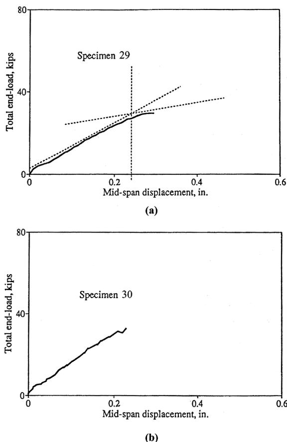
Fig. 5—Load-displacement response of specimens: (a) Specimen 29; and (b) Specimen 30.
