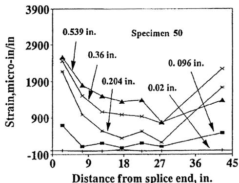
Fig. 10—Strain in stirrups placed over splice region: Specimen 50.
