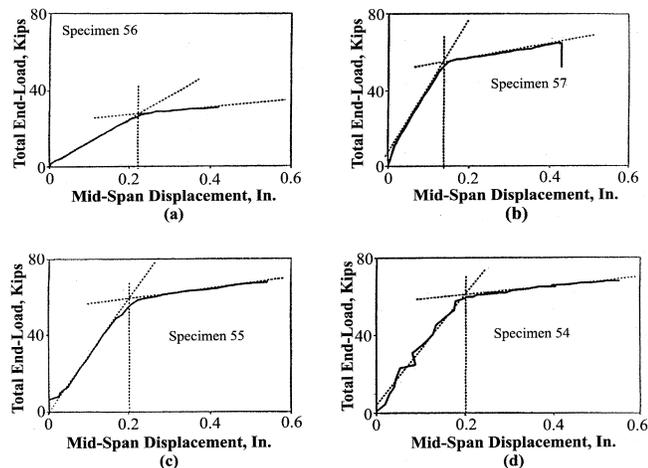
Fig. 7—Load-displacement response of specimens with stirrups: (a) Specimen 56; (b) Specimen 57; (c) Specimen 55; and (d) Specimen 54.
