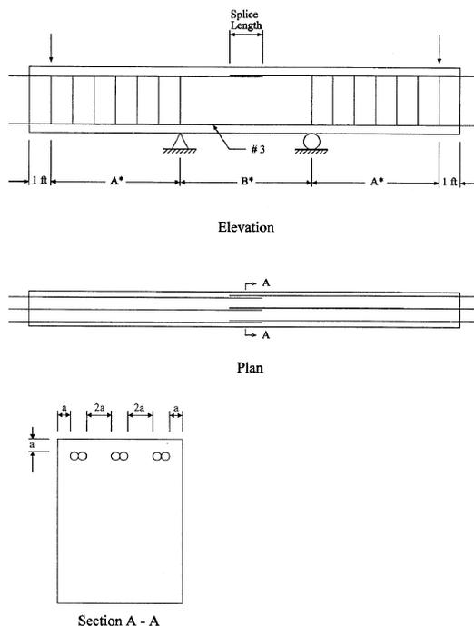
Fig. 1—Test specimen.
