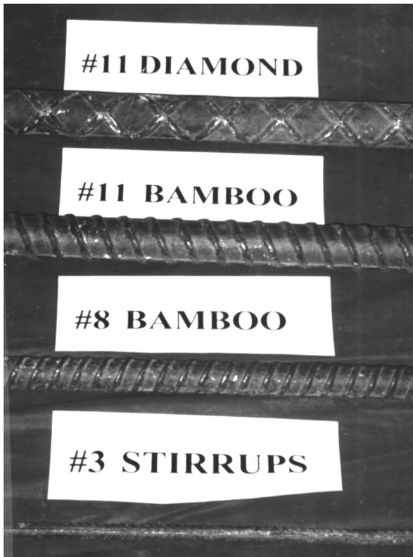
Fig. 2—Different bar sizes used in experimental program.
