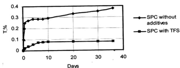
Fig. 2 Change of shrinkable deformations T (%) during hardening of SPC.
