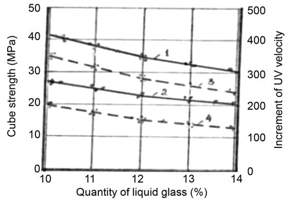
**Fig. 1** Change of strength and density of SPC depending on the consumption of the liquid glass: 1-Change of SPC strength with the TFS additive, 2-Same without the additive, 3-Change of US velocity into SPC mix with the TFS additive, 4-Same without the additive.
