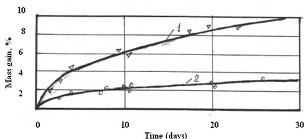
Fig. 3 Change of weight of SPC samples in water: 1-composition modified by FA; 2-same but by TFS.
