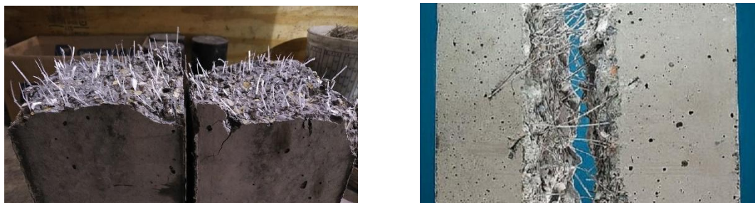
Fig 1.1: Fiber reinforced Concrete
