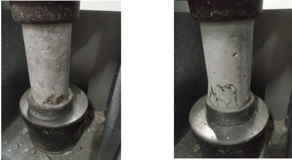
Fig 5.18: 0.5% fiber (Compressive strength failure pattern) at 200°C
