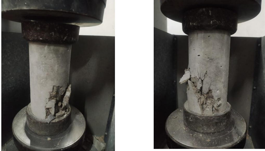
Fig 5.16: 0 % fiber (Compressive strength failure pattern) at 200°C
