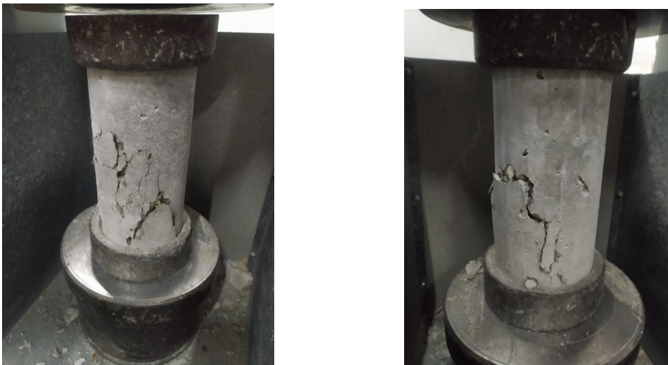
Fig 5.19: 0.75% fiber (Compressive strength failure pattern) at 200°C
