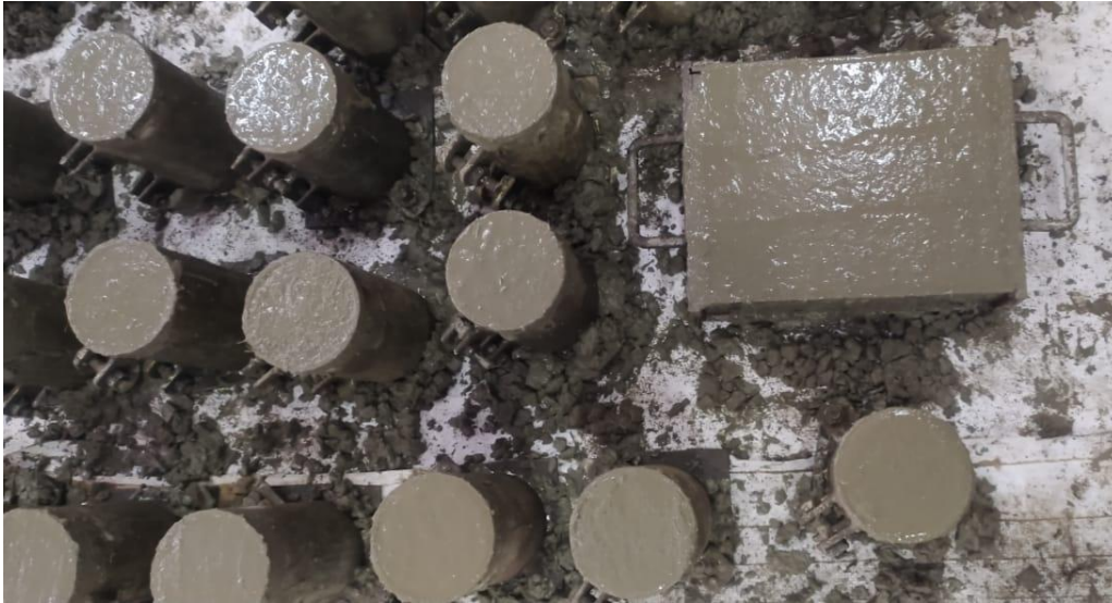
Fig 4.9: Concrete casting in mold
