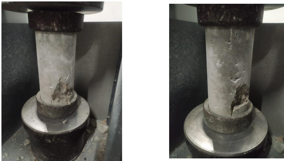
Fig 5. 17: 0.25 % fiber (Compressive strength failure pattern) at 200°C
