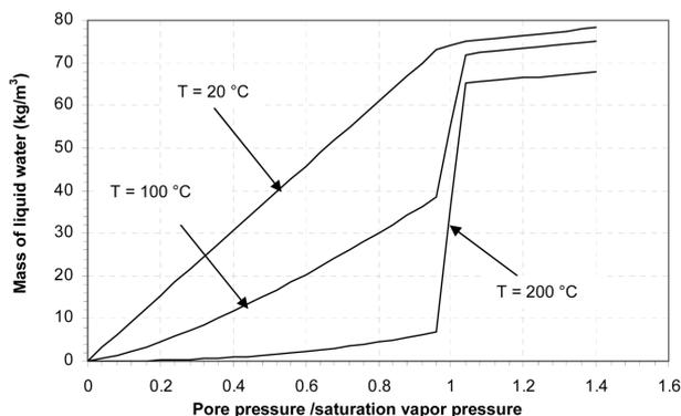
Fig. 8 Isotherms for HSC used in the analysis.
