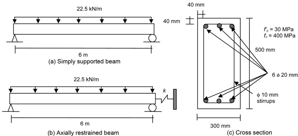
**Fig. 2** Cross section and elevation of RC beam used in parametric studies.
