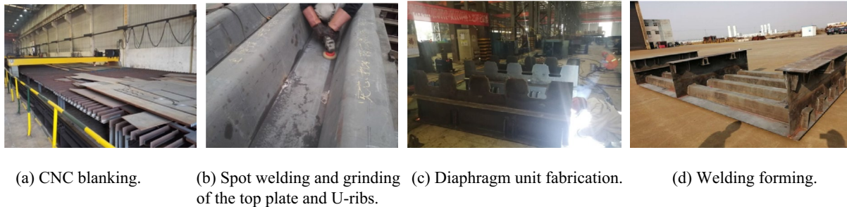
Fig. 14 Main manufacturing process of the laboratory-test specimen pieces
