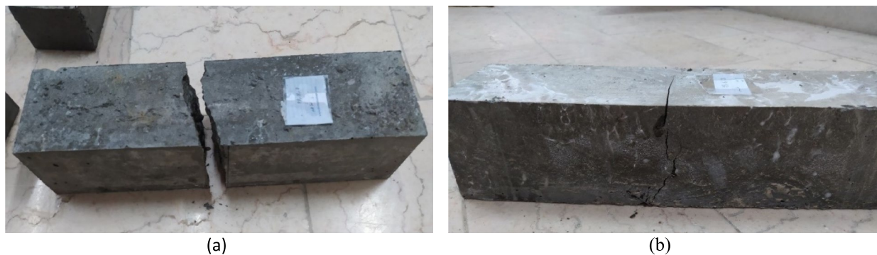
Fig. 15 Failure appearance of concrete samples in flexural strength test a without fiber; b with steel fiber
