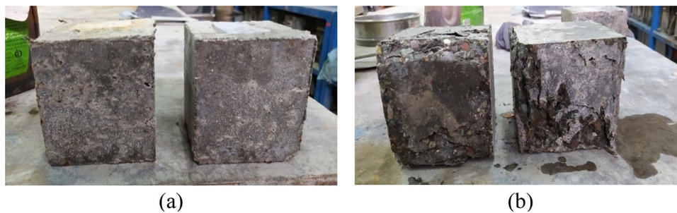
Fig. 20 Appearance of concrete with steel fiber in compressive strength a before testing; b after testing
