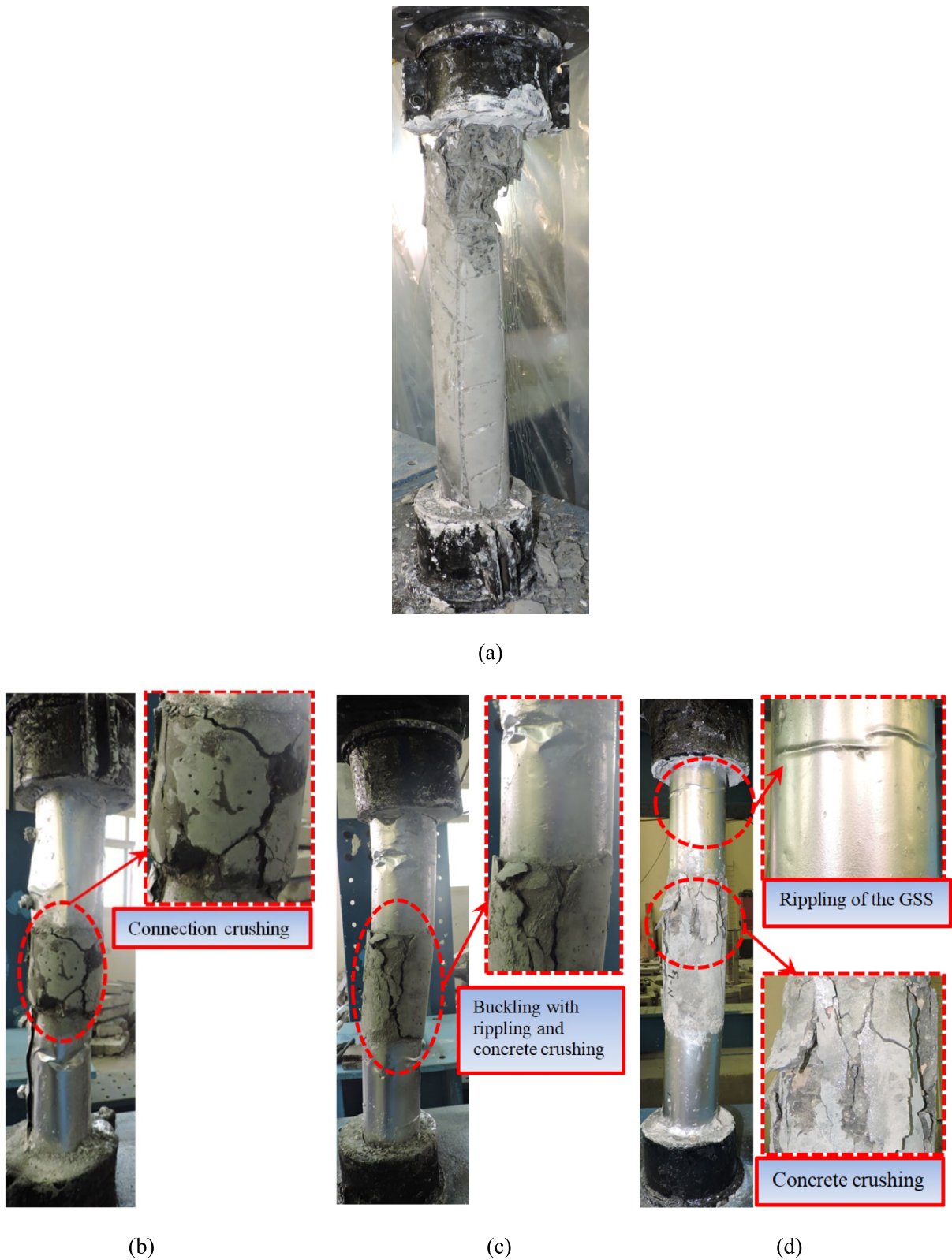
Fig. 5 Failure mode of the tested columns: a Column C0, b Column N-L1, c Column N-L2, d Column N-L3, e Column E-L1, f Column E-L2, g Column E-L3, h Column H-L1, i Column H-L2, and j Column H-L3
