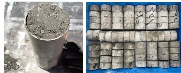
(a) Concrete pouring (b) Specimen cutting Fig. 2 Schematic diagrams of cylindrical specimen preparation
