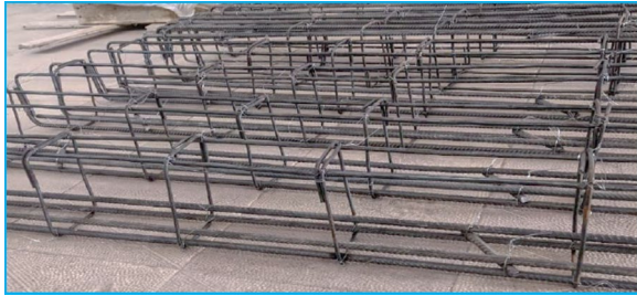
Fig. 5 Reinforcement details of the tested beams
