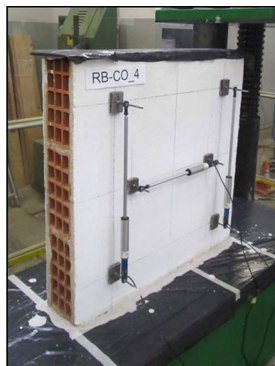
Fig. 16 Vertical compression test method of wallette. Reprinted from Minotto et al., (2020)
