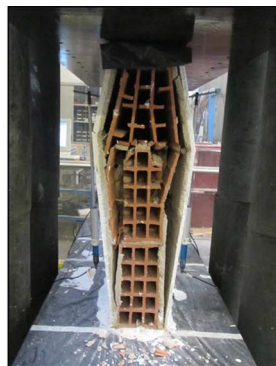
Fig. 16 Vertical compression test method of wallette. Reprinted from Minotto et al., (2020)
