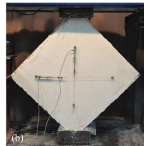
Fig. 17 Diagonal compression test method of wallette. Reprinted from Gkournelos et al., (2020)
