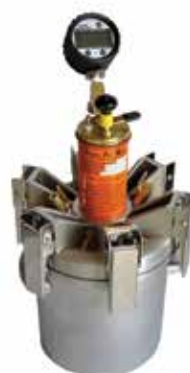
Fig. 4: The sequential air method (SAM) meter (photo courtesy of Tyler Ley, Oklahoma State University)
