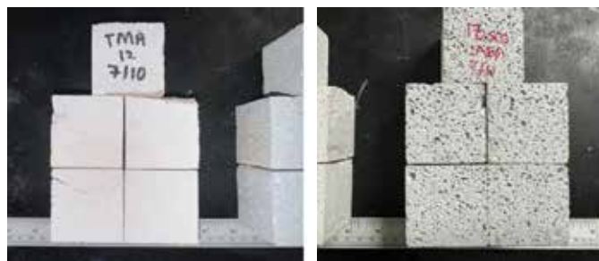
Fig. 6: AAC made using conventional metallic aluminum powder (left) and AAC made using MSWI BA (right)
