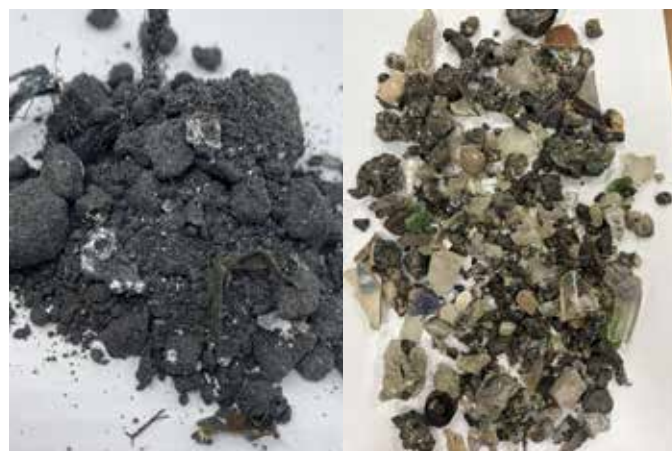
Fig. 1: MSWI BA fresh (left) and washed (right)
