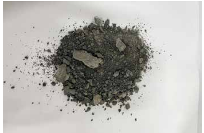
Fig. 8: MSWI ash-amended clinker created using 1 to 2% MSWI BA addition to the cement kiln feed
