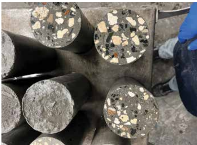
Fig. 2: Test cylinders with MSWI BA as aggregate
