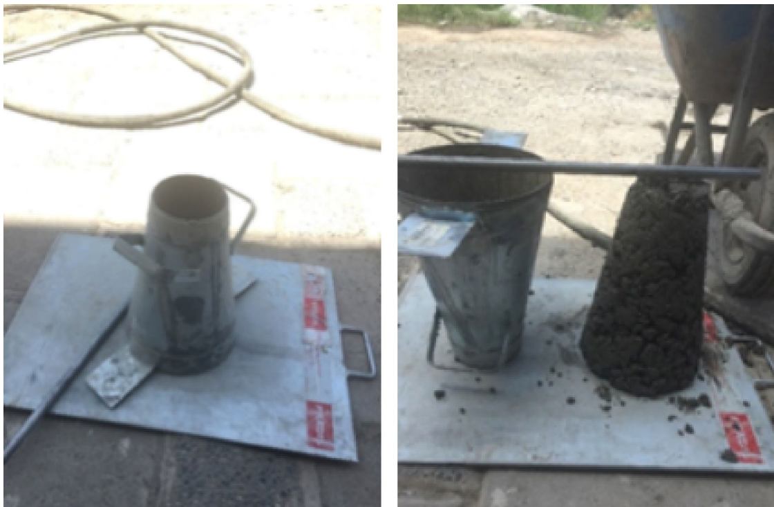
Fig. 3 Abrams cone test for determining the workability of concrete samples
