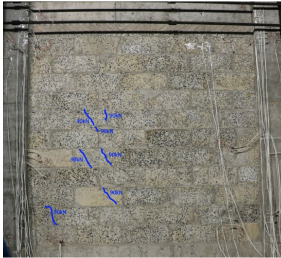
Fig. 13 First cracks at 90 kN. The blue lines were cracks of horizontal load at 90 kN, and light green lines at 100–140 kN, and yellow lines at 150–180 kN, and pink lines at 200–250 kN, and red lines at 280 kN
