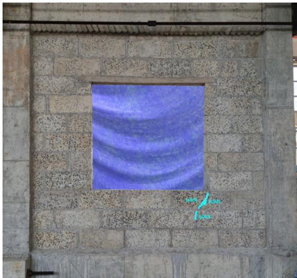
Fig. 11 First cracks at 60 kN. The lake blue lines were cracks of horizontal load 60 kN, the blue lines for 70–80 kN, the green lines for 100–140 kN, the yellow lines for 160–180 kN and the pink lines for 200–280 kN
