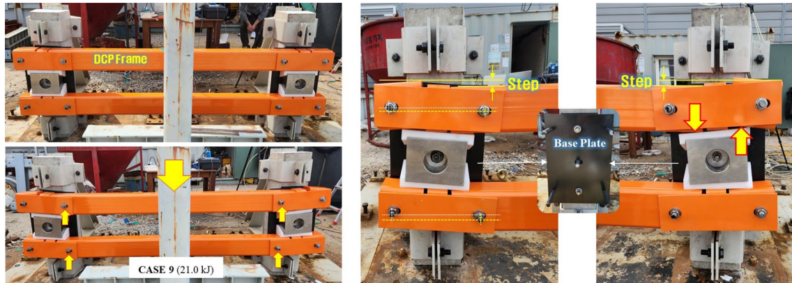
Fig. 16 Specimen appearance post-impact (Case 9)
