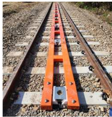
Fig. 6 Steel frame grid type DCP of ballasted track (DCP Type 1)
