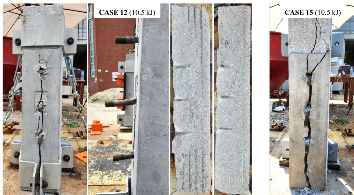
Fig. 19 Damage to sleeper and buried anchors post-impact (Cases 12 and 15)
