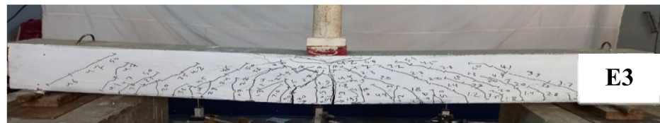
a) Experimental crack pattern
