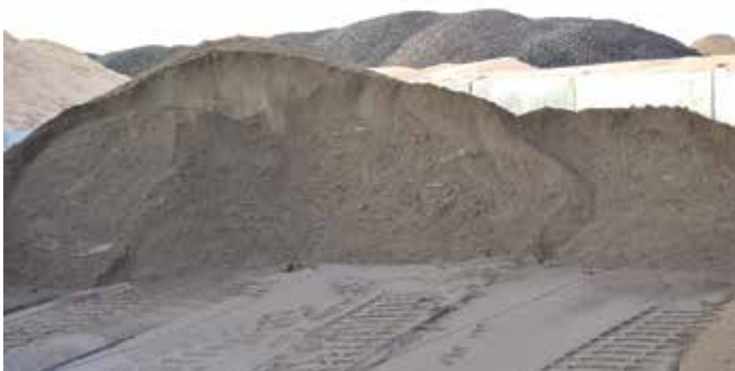
Presoaked lightweight aggregate ready for batching (photo courtesy of the Expanded, Shale, Clay and Slate Institute)
