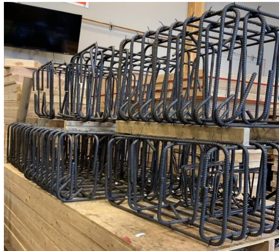
Figure 4.6. Reinforcement Cages for Top and Bottom Blocks
