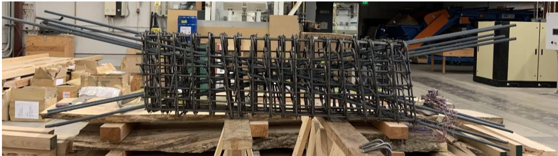
Figure 4.8. Reinforcement Cage for D(#4)-3.0-0.69 or D(#4)-3.0-1.38
