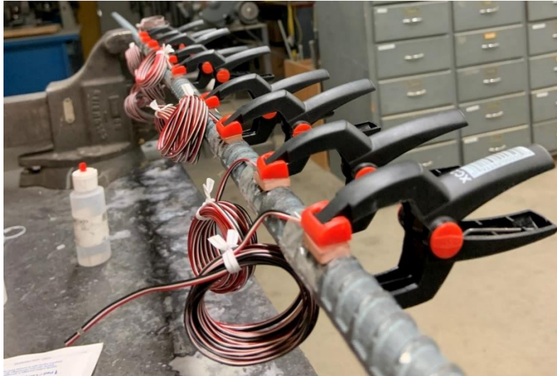
Figure 4.5. Strain Gauge Installation
