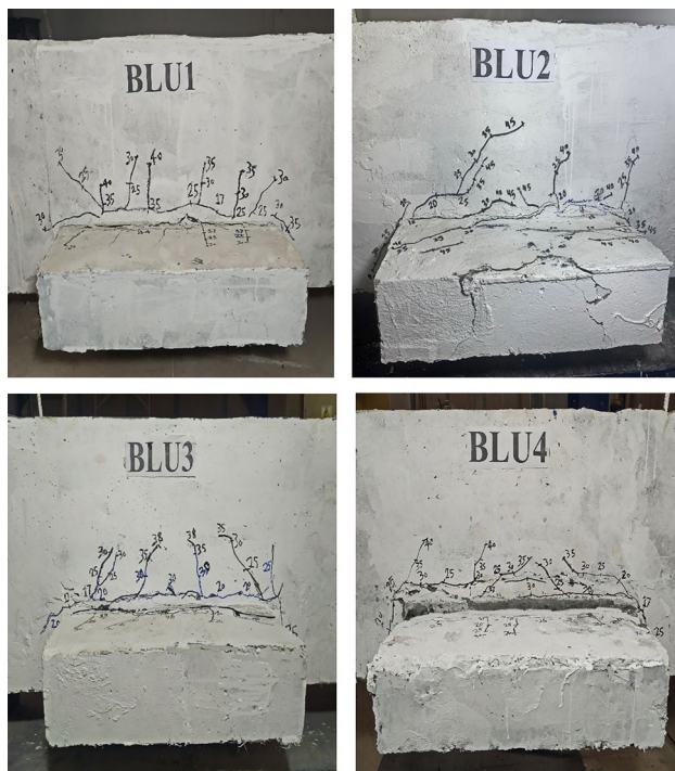
Fig. 5 Failure modes and crack patterns for BLU1, BLU2, BLU3, and BLU4 (note: the loads marked on the specimens are in tons)
