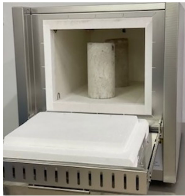
Fig. 1 Heating test of the concrete specimen
