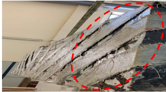
c) Separation (debonding) of the GFRP strips (beams B 2,1,100,100,45 and B 4,1,150,100,60 ).
