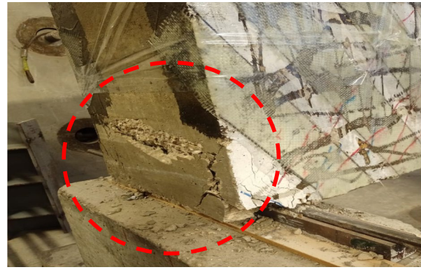
b) Failure at the support region (bearing failure mode) (beams B 1,1,150,100,45 , B 1,3,150,100,45 , B 1,2,150,100,45 , B 3,1,150,125,45 , B 4,1,150,100,90 , and B 3,1,150,75,45 ).
