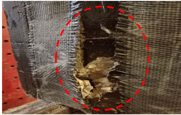
a) Concrete cover separation (beam B 2,1,200,100,45 ).
