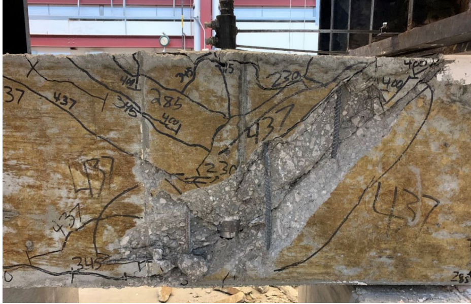
Figure 5.24 Anchorage failure observed in specimen 14-16E ( A_{tt}/A_{hs} = 0.551 )
