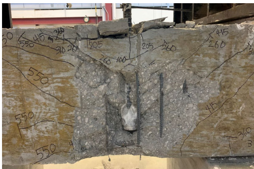
Figure 5.23 Anchorage failure observed in specimen 14-16D ( A_{tt}/A_{hs} = 0.827 ) tested under loading condition A (after removal of loose concrete)
