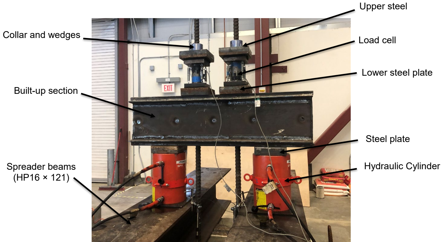
Figure 2.14 Test frame – second configuration
