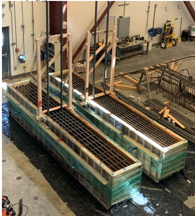
Figure 2.10 Horizontal formwork for No. 18 bar specimens
