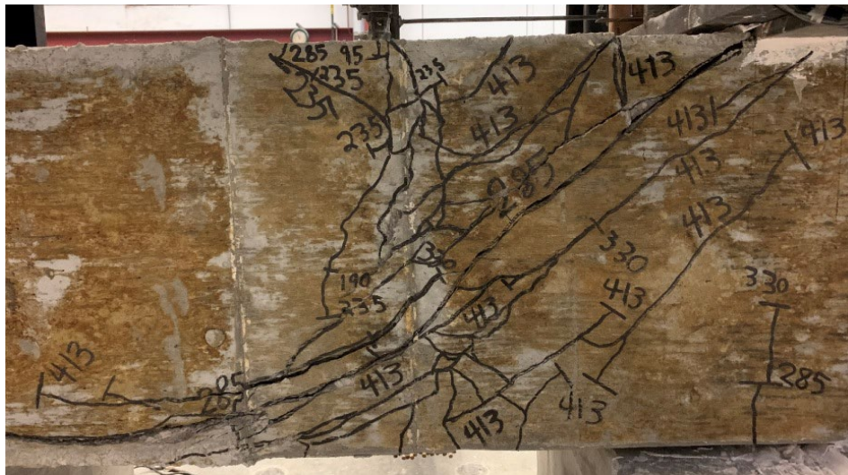
Figure 5.29 Concrete breakout observed in specimen 14-17 ( A_t/A_{hs} = 0.551 ) with increased side cover to the bar and decreased bar spacing
