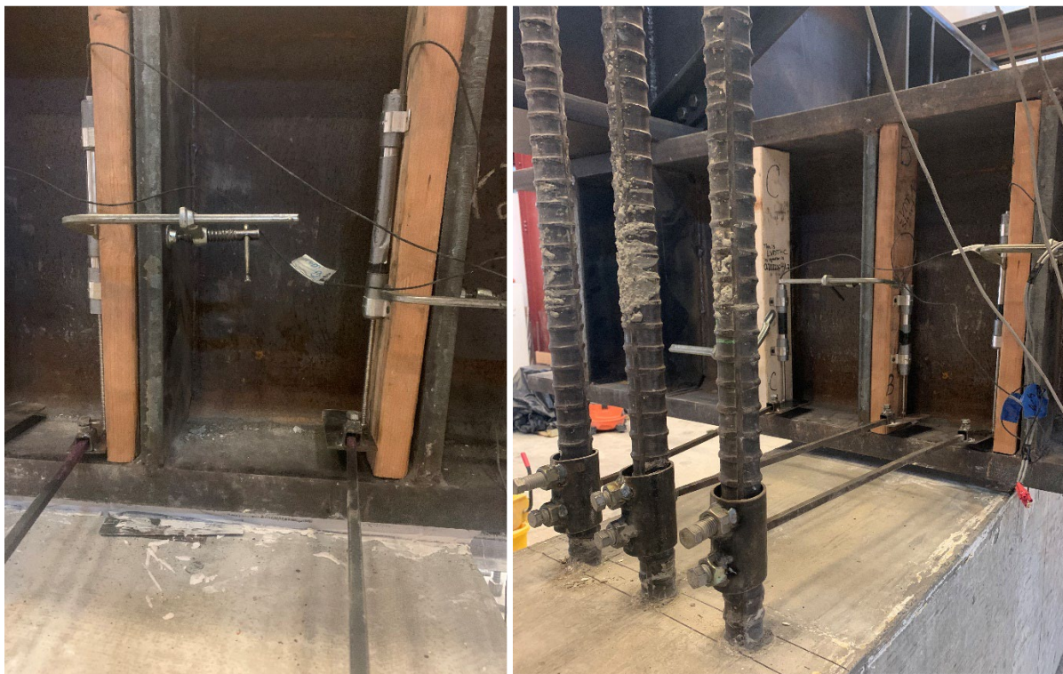
Figure 2.22 Setup for using the LVDTs
