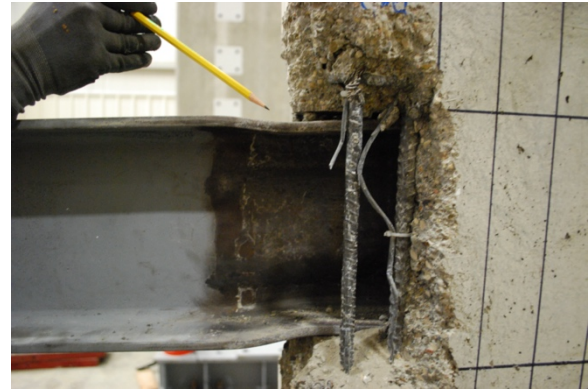
Figure 3.20 Damage at the conclusion of wind load protocol testing (loose concrete was not removed) – specimen 2b (test 4).
