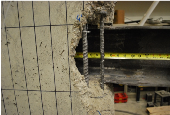
Figure 3.20 Damage at the conclusion of wind load protocol testing (loose concrete was not removed) – specimen 2b (test 4).
