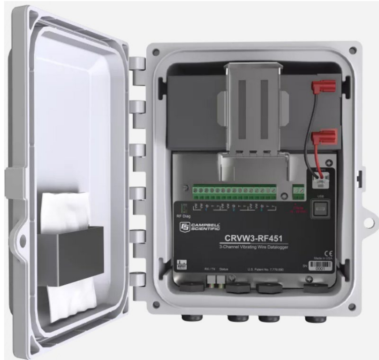
Figure 10: Campbell Scientific CRVW3 Datalogger
