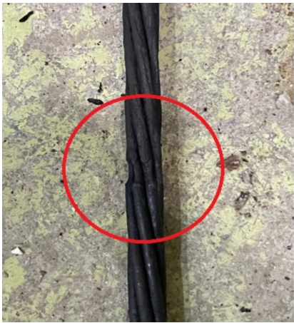
Fig. 10 Cross section of a corroded prestressing strand
