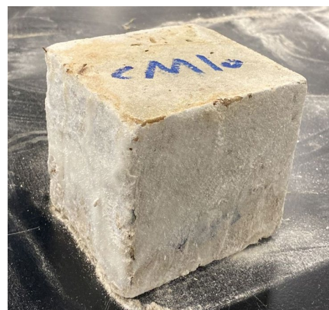
Fig. 4 Concrete mixture appearance after exposure to an acidic environment before testing
