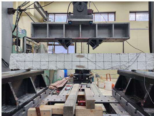
(B) Photo of the flexural test setup
