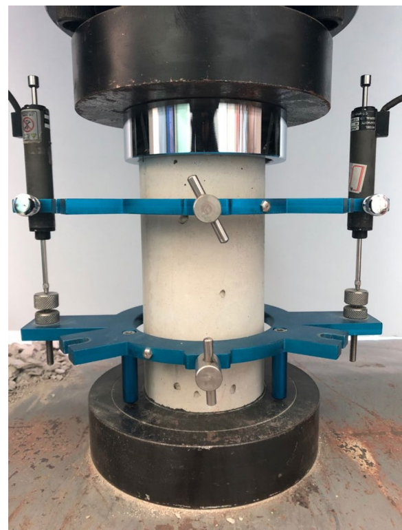
Fig. 4 Concrete compressive strength test setup
