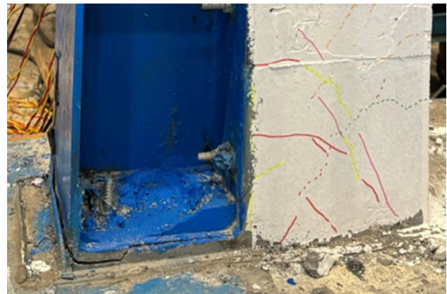
Fig. 8 End plate of H -shaped steel warping ( R=1.0\% )
