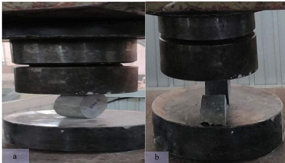
**Fig. 12** Splitting tensile strength (Brazilian test) for cement sheath compositions **a** before applying axial compressive failure load; **b** after applying axial compressive failure load
