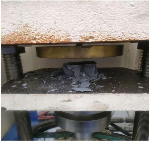
**Fig. 11** Load frame for destructive CS measurements
