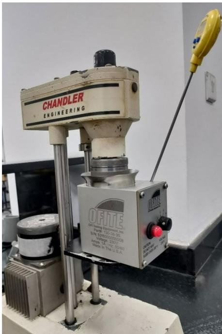
**Fig. 4** Rotational viscometer for slurry rheological parameters measurements
