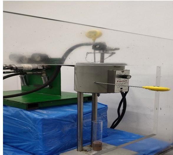
**Fig. 8** Non-stirred fluid loss apparatus for slurry filtrate volume measurements
