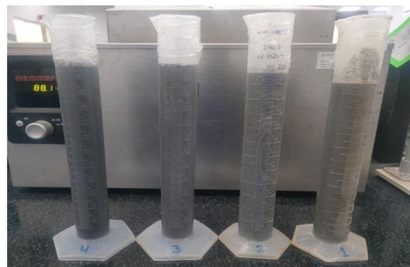
**Fig. 5** 250-mL graduated cylinder for API 10B-2 slurry free fluid measurements
