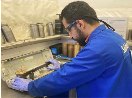
**Fig. 3** Pressurized mud balance for slurry density measurements
