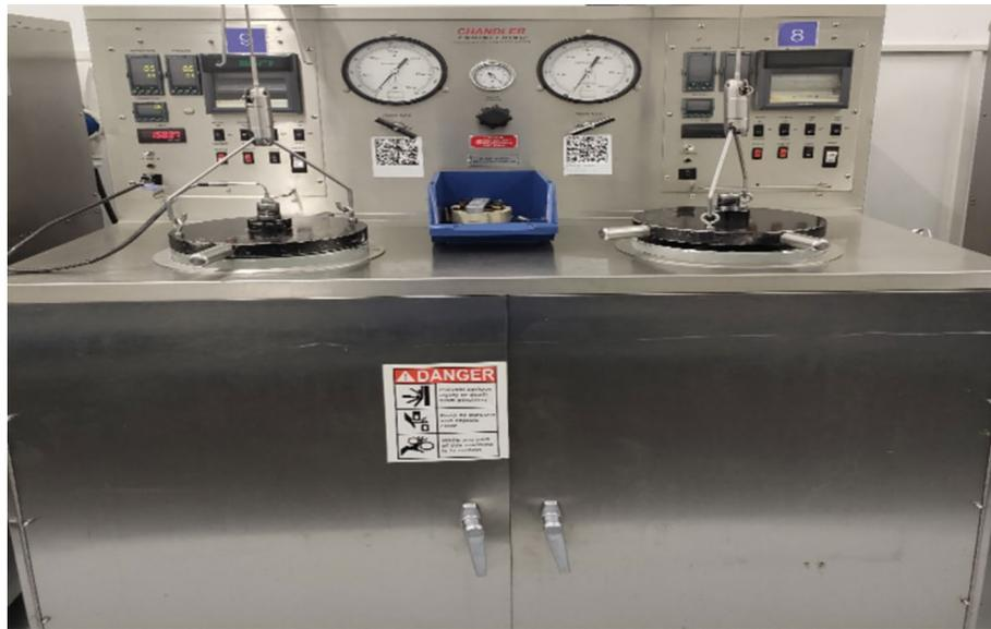
**Fig. 9** HPHT consistometer for slurry thickening time measurements
