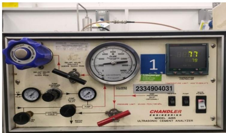
**Fig. 10** Ultrasonic cement analyzer for nondestructive CS measurements
