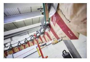
accurately conveys each bag from the RADIMAT to a single-bag feeder at the end of the line, which then places each bag precisely onto the packing machine's filling spouts. The PATHFINDER Edition can also be implemented in a simplified version without the use of a RADIMAT. Rather than having to place the bag on the actual spout, operators simply feed the bags into the conveying system itself, which then applies the bag to the spout automatically.
