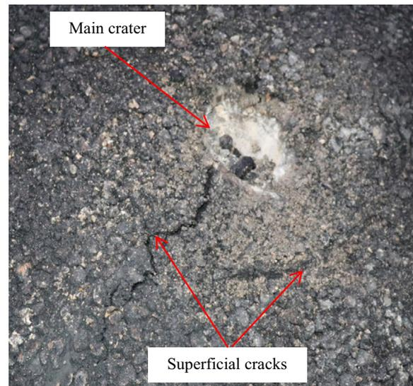
Fig. 13 Superficial cracks initiating along the top surface of SR30F0, SR40F0, and SR50F0 slabs
