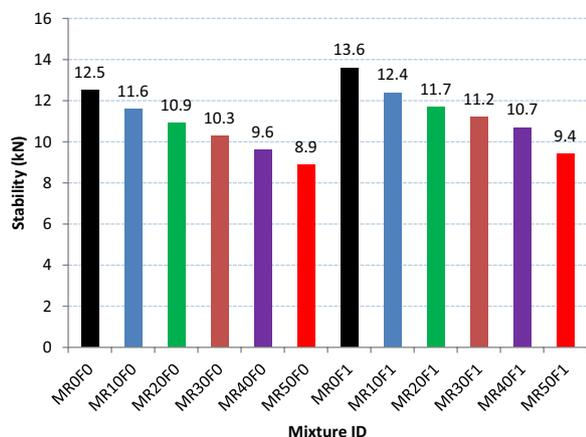
**Fig. 7** Effect of RCA ratio and corrugated steel fibers on Marshall stability
