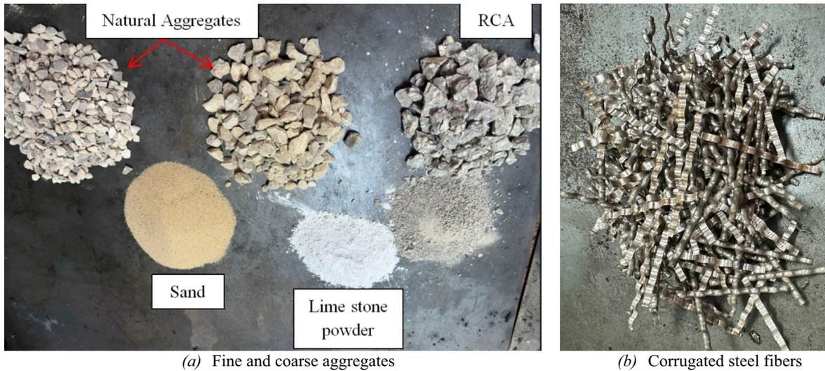
**Fig. 2** The materials used in casting mixtures. **a** Fine and coarse aggregates. **b** Corrugated steel fibers
