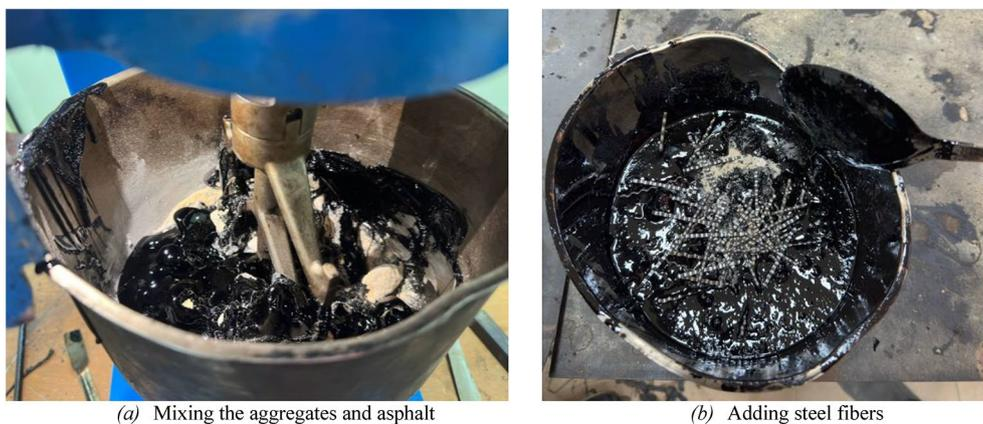
**Fig. 3** Mixing the components of asphalt mixtures. **a** Mixing the aggregates and asphalt. **b** Adding steel fibers
