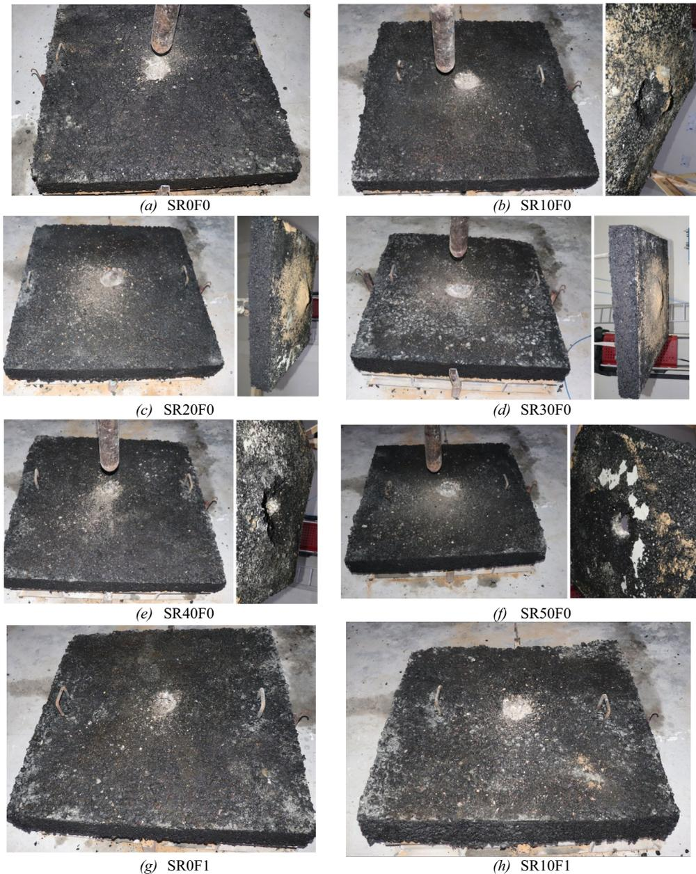
**Fig. 12** Failure patterns of asphalt slabs subjected to impact loads
