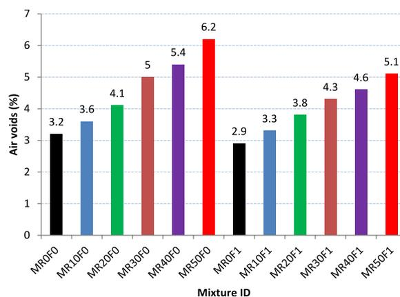
Fig. 10 Effect of RCA ratio and corrugated steel fibers on air voids of asphalt mixtures
