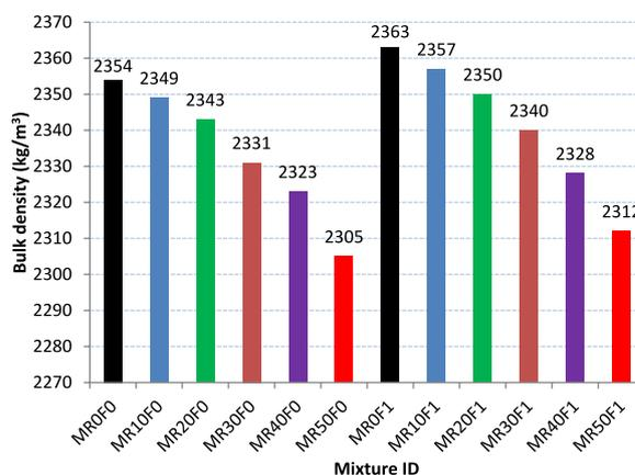
**Fig. 9** Effect of RCA ratio and corrugated steel fibers on bulk density of asphalt mixtures
