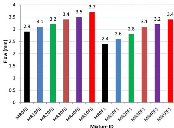
**Fig. 8** Effect of RCA ratio and corrugated steel fibers on Marshall flow
