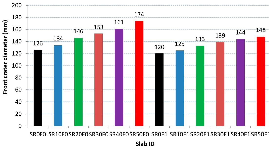
**Fig. 14** Effect of RCA ratio and corrugated steel fibers on front crater diameter of asphalt slabs
