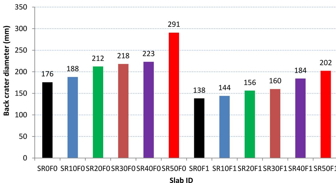
**Fig. 15** Effect of RCA ratio and corrugated steel fibers on back crater diameter of asphalt slabs
