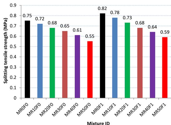
**Fig. 11** Effect of RCA ratio and corrugated steel fibers on splitting tensile strength of asphalt mixtures
