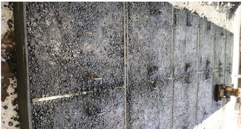
**Fig. 5** Preparation of asphalt slabs
