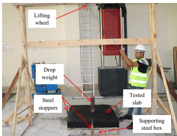
**Fig. 6** The manual free fall impact test equipment
