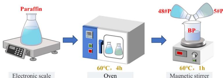
Fig. 1 The preparation flowchart of BP
