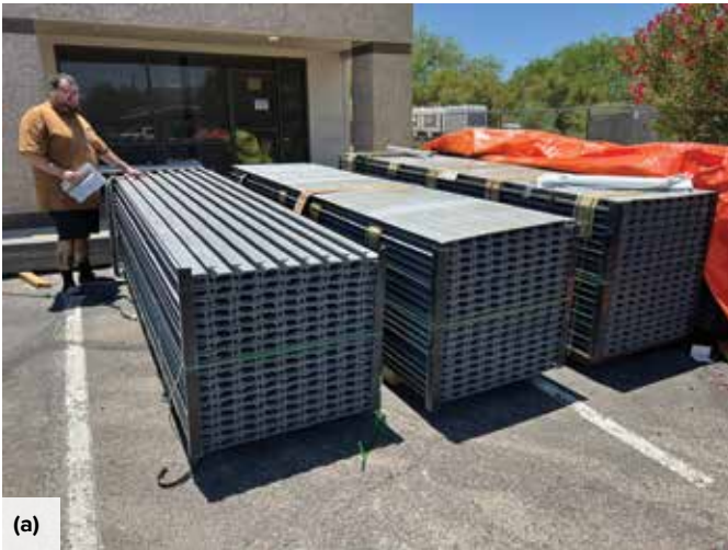
Fig. 2: T-panels: (a) 3 ft (910 mm) wide and 12 or 18 ft (3.7 to 5.5 m) long; (b) close view of grit coated surface and steel reinforcing bars that would provide equivalent tensile capacity
