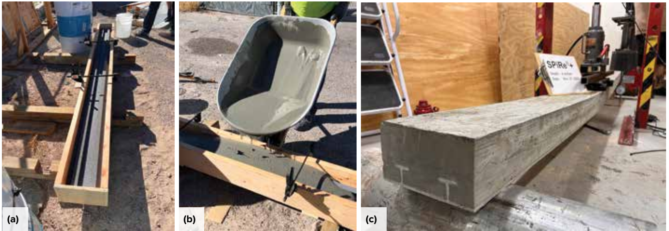
Fig. 3: Test specimen: (a) formwork; (b) mixing and placement of grout; and (c) flexural testing of the beam
