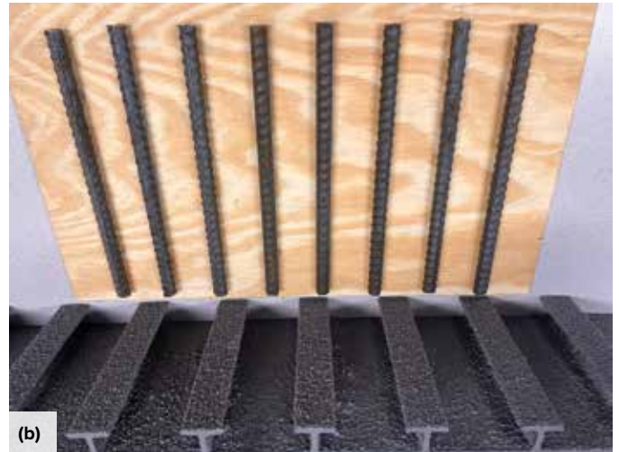
Fig. 2: T-panels: (a) 3 ft (910 mm) wide and 12 or 18 ft (3.7 to 5.5 m) long; (b) close view of grit coated surface and steel reinforcing bars that would provide equivalent tensile capacity
