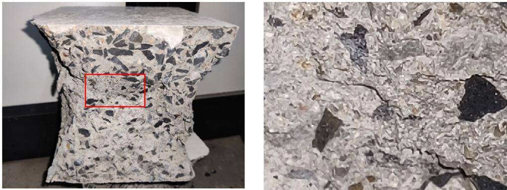
**Fig. 7** Sample representation for mortar failure mode (cracks propagating through mortar)
