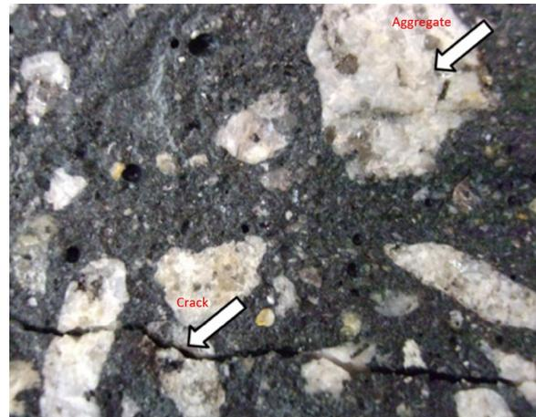
**Fig. 6** Aggregate failure mode (crack going through aggregates)—adapted from Zhang and Islam (2012)
