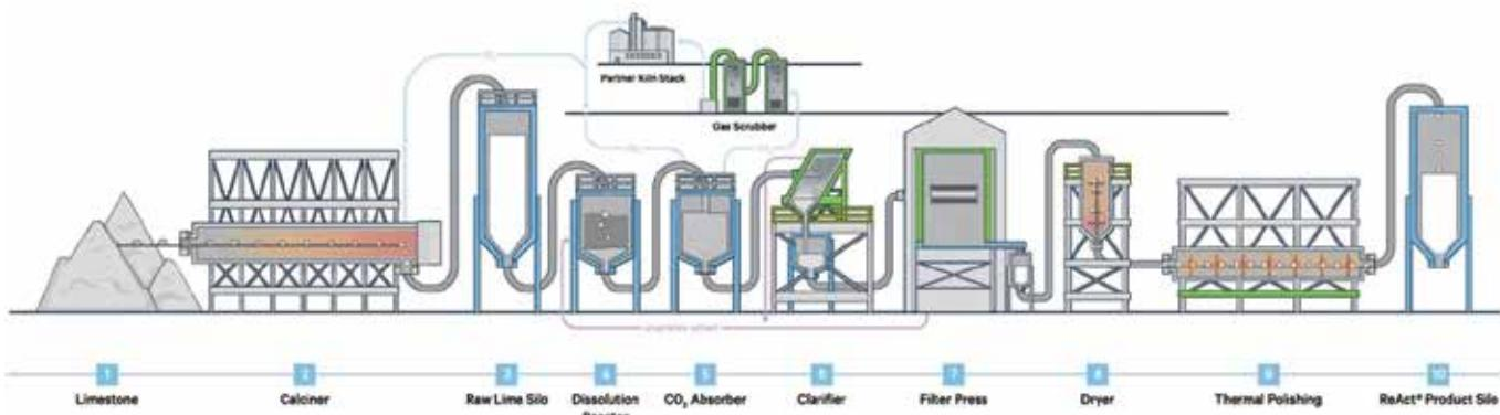
Fig. 1: Fortera's process produces reactive calcium carbonate by dissolving lime in a proprietary solvent, bubbling CO<sub>2</sub> through the solution, and processing the resulting precipitate
