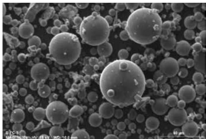
**Fig. 2: The Terra CO<sub>2</sub> process is based on vitrification of silicates. The company is currently producing a glassy, microspherical pozzolanic supplementary cementitious material and is developing a nonhydraulic binder**
