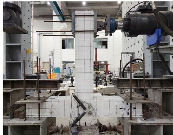
**Fig. 5** Testing frame, boundary conditions and LVDT positions of PJ-CU specimen
