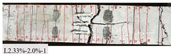
**Fig. 2** Example of multiple cracking and localized crack in this study
