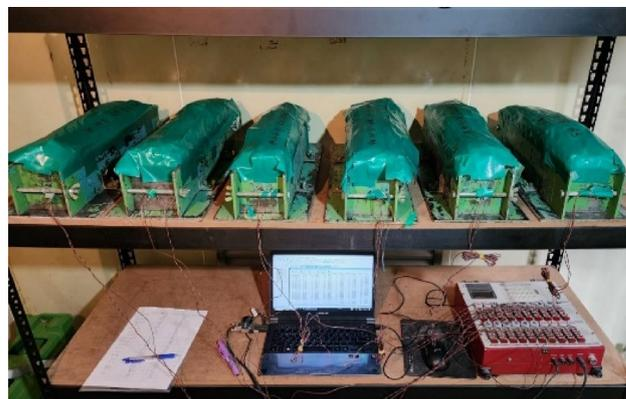
**Fig. 4** Autogenous shrinkage test setup: Modified from KS F 2586: 2021. (a) Cross-section of a shrinkage test specimen. (b) Autogenous shrinkage test and measurement under progress Additional name for Fig. 4
