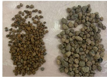
**Fig. 3** Structure of the synthetic-based lightweight LECA grains
